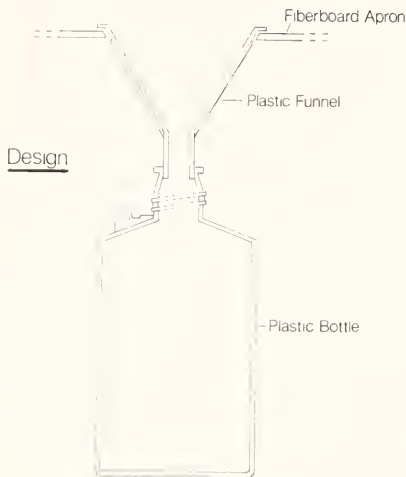
Fig. 1. Design and placement of large capacity pitfall trap.
