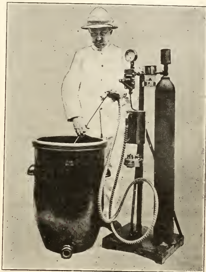
WILHELM PAHL'S RAPID COAGULATOR FOR Hevea LATEX BY CARBONIC ACID.
