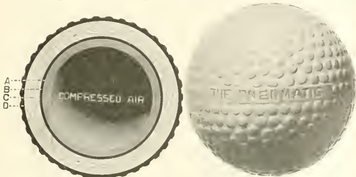
[A—Air retainer. B—Jacket for air retainer. C—Wound fiber wall. D—Tough cover.]
