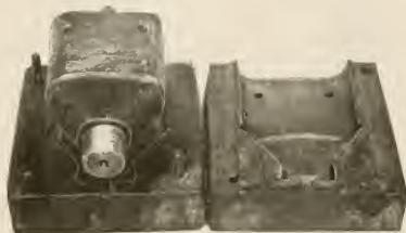
FIG. 1. HOT WATER BOTTLE FUNNEL SHAPING MOLD AND CORE.
