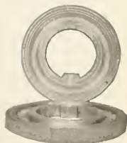
FIG. 7. AEROPLANE TIRE INNER TUBE PRESS MOLD.
