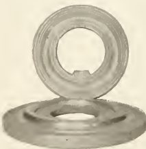
FIG. 6. AEROPLANE TIRE INNER TUBE SHAPING MOLD AND CORE.
