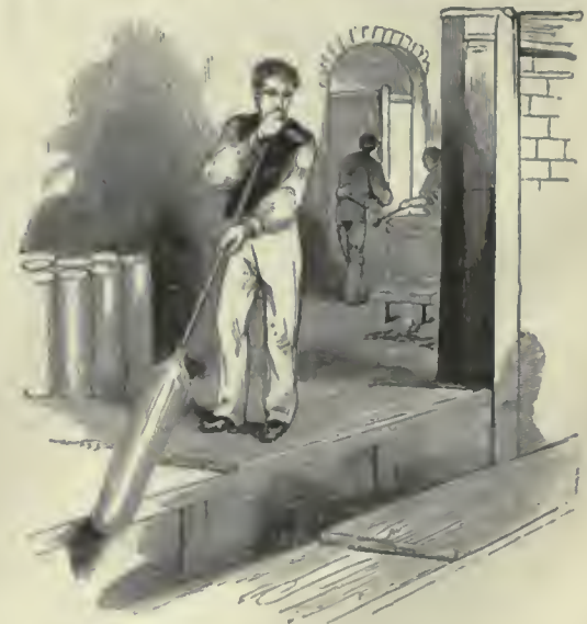
Swinging and blowing Sheet-glass.
