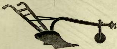
2248. Moldboard view of a steel moldboard walking-plow showing beam wheel.
