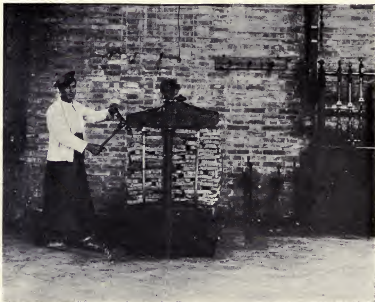
FIG. 1118.—Baling cork after boiling, scraping, grading and trimming. Considerable cork is shipped to this country in this form. Photograph taken at a large cork factory in Seville, Spain.
