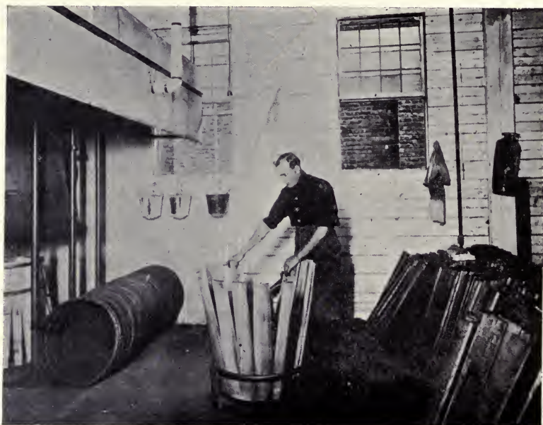
FIG. 32.—First step in assembling a barrel.
