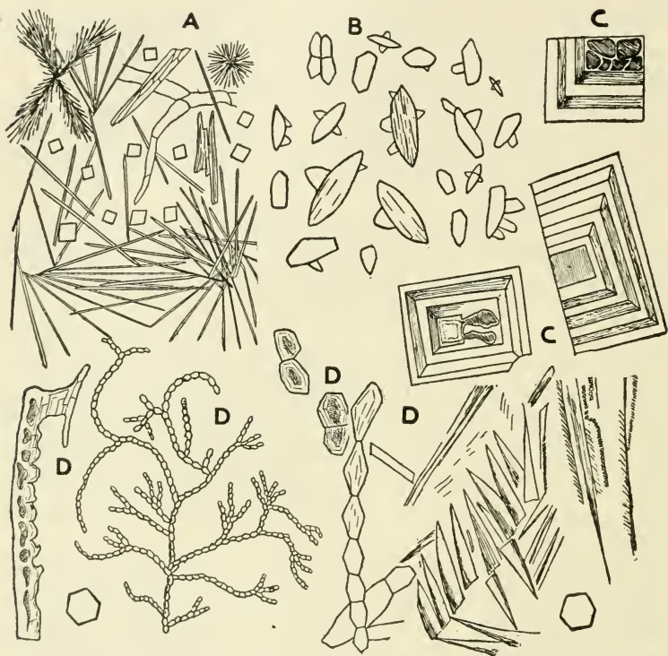
FIG. 419. Crystals of some of the common reagents which not infrequently separate on the slide and may be mistaken for cell contents: A, isotropic crystals of chloral which occur in cubes about 10\ \mu in diameter or long needles about 50\ \mu long; B, phloroglucin which occurs in broad rectangular plates or ellipsoidal discs from 10 to 35\ \mu in diameter which are doubly refracting with a play of colors; C, cubes of potassium iodide which are isotropic; D, crystals from potassium hydrate solution which separate in broad prisms and branching chains that are doubly refracting and give marked color effects.
