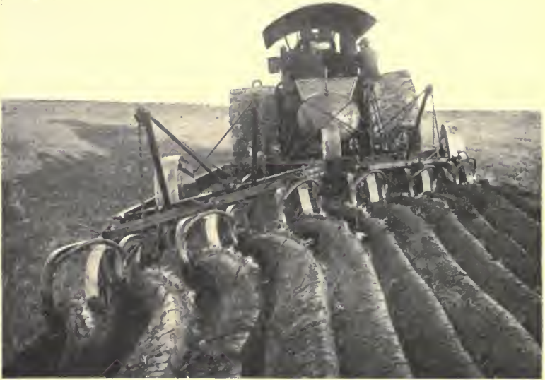
FIG. 75. Modern steam gang plow
