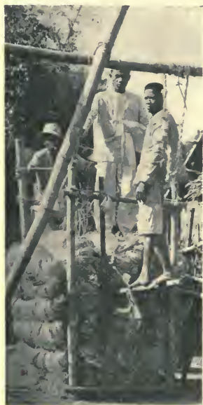
FIG. 96. Primitive abacá press in Albay
