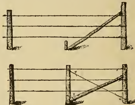
1726. Illustrating the bracing of the end post in a fence or trellis.
