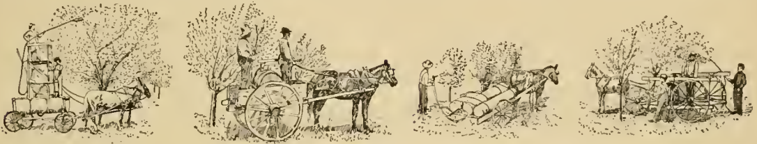
1594. Various spraying rigs. 1. A tall platform rig, to enable one to spray very high trees. 2. A simple barrel outfit for small orchards and small trees. 3. Compressed air outfit. 4. A low rig, with barrel. For larger machines, and other patterns, see pages 1058-1060 (Vol. II).
