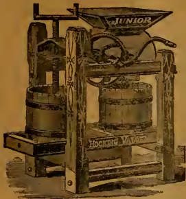
Cider Mills—with wooden crushing rollers.
