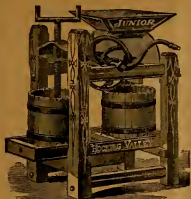
Cider Mills—with wooden crushing rollers.
