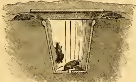
Section of an effective Mole-trap.
