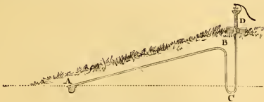
Pumping Water up a Slope.
