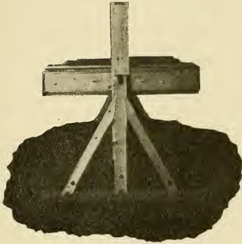
FIG. 6. End view of table. Note heavy construction of base; central point on which the whole egg containing portion of the table turns.
