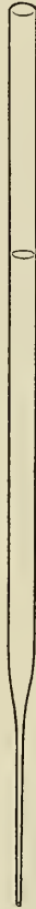
FIG. 30—Capillary pipette. A piece of glass tubing drawn to capillary size at one end. Reduced to three-fourths of the size used. (Original.)
