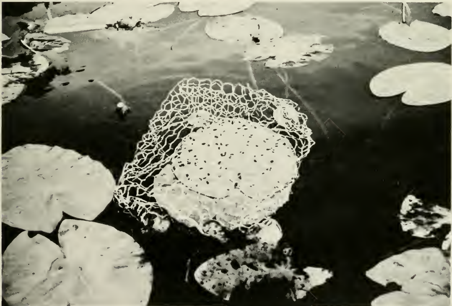
Fig. 2. Lime-trap for insects. For explanation, see text. The wire netting is kept floating by corks and is attached with a string to the petiole.
