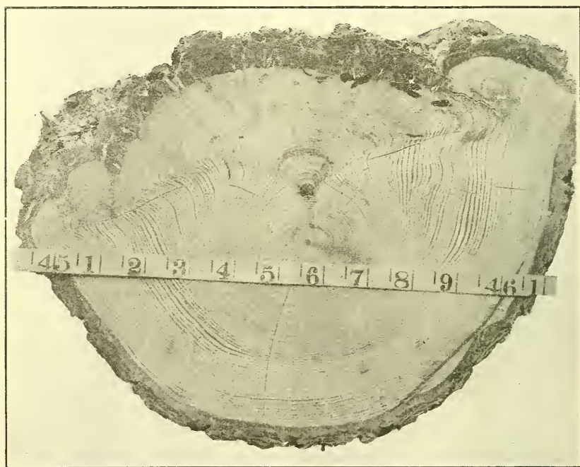
FIG. 23.—Cross section of one of the burls on the Douglas fir shown in figure 22. This section does not pass through the point showing the age at which the infection first occurred. (The tape shows feet in tenths.)
