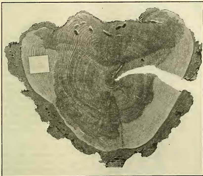
FIG. 24.—Cross section of a burl on a western larch caused by Razoumofskya laricis . Diameter of burl, 2 feet. Note the presence of borers and fungi. The check appeared in seasoning.
