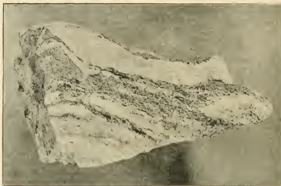
FIG. 1.—Block of Gneiss, twenty centimetres long, from Co. Mayo, showing (i) curving upper surface formed by fracture along a foliation-plane; (ii) dissimilar materials in different bands, the lighter ones consisting of quartz and felspar, and the darker ones being rich in dark mica; (iii.) a lenticular mass at the right-hand end, with the darker layers flowing round it.
