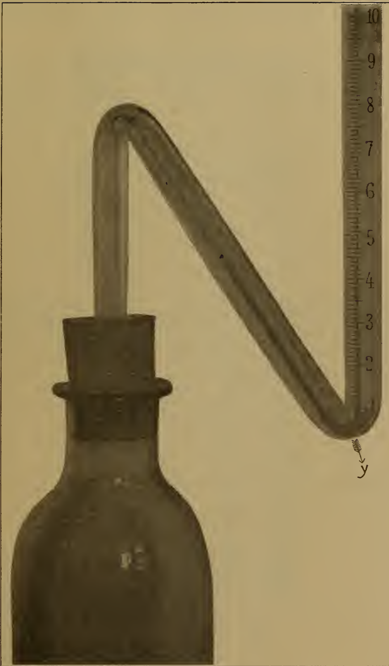
FIG. 9.—Detail picture of the outflow tube and piezometer.
