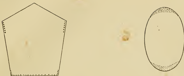
Fig. 1.—Showing diagrammatically by dots where grain is affected when stored in a Morai (left) or Pura (right).
