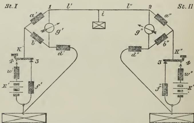
It has also been proposed to use Ruhmkorff's coils for balancing the effect of charge and discharge. This method, however, I believe must be always much inferior to the one of using condensers, inasmuch as the strength of a Voltaic induction current scarcely depends on the speed of signalling, while the charge and discharge of a line, it is well known, is not at all an inconsiderable function of the signalling speed.
