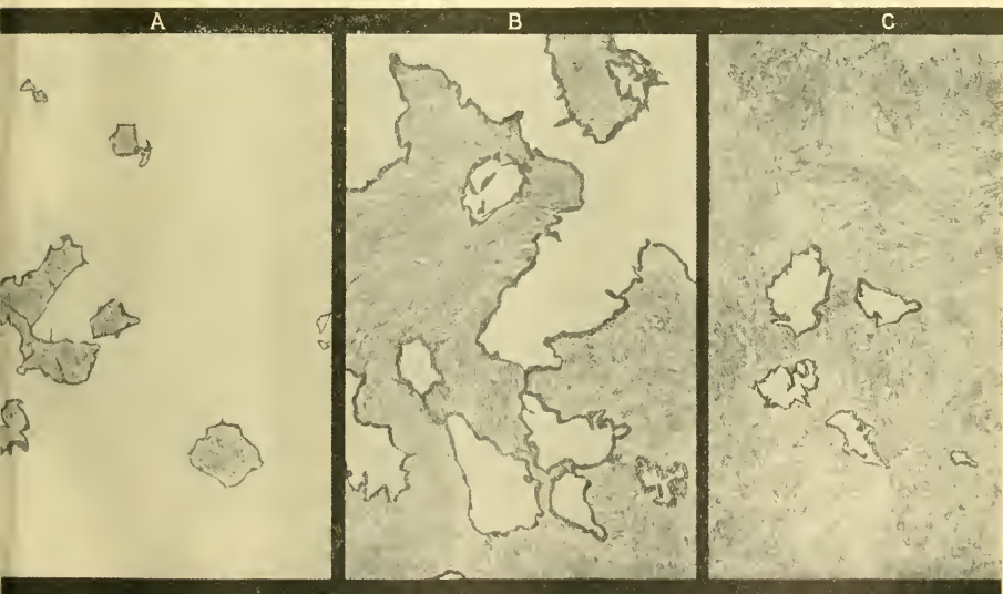
Transformation nearly completed. Temperature about 730^{\circ}\text{C} . Transformation half completed. Temperature about 725^{\circ}\text{C} . Transformation beginning. Temperature about 723^{\circ}\text{C} . 10. 3.—Pale areas, hardenite. Laminated areas, normal pearlite. Dark borders, troostitic pearlite. [Carbon 0.89 per cent. Magnified about 450 diameter.]
