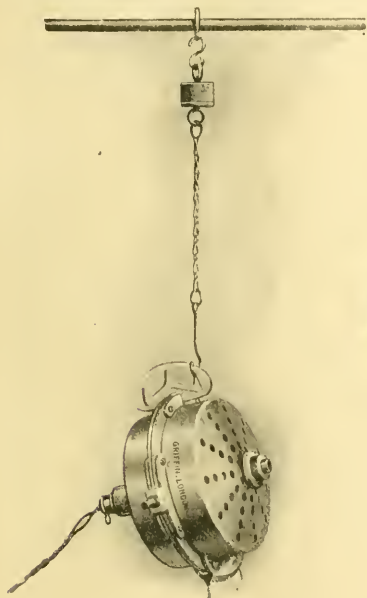
FIG. 8.—Motor-gyrostat precessing on chain support.
