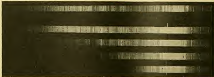
FIG. 1.—1. Spark spectrum of nickel and iron. 2. The same, after the light has passed through quartz 10 mm. thick. 3. Crown glass 0.13 mm. thick. 4. Crown glass 0.33 mm. thick. 5. Window glass 1.62 mm. thick.
