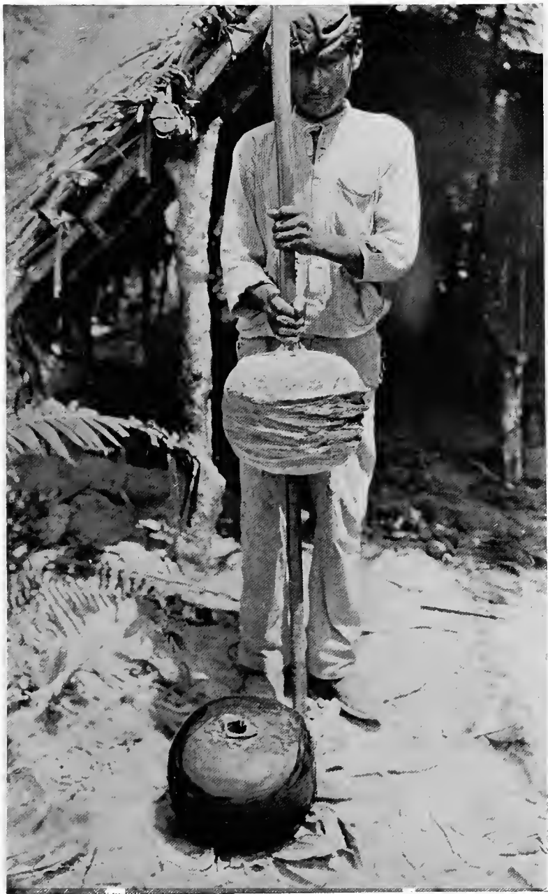
REMOVING THE BALL OF RUBBER AFTER IT HAS BEEN SMOKED.
