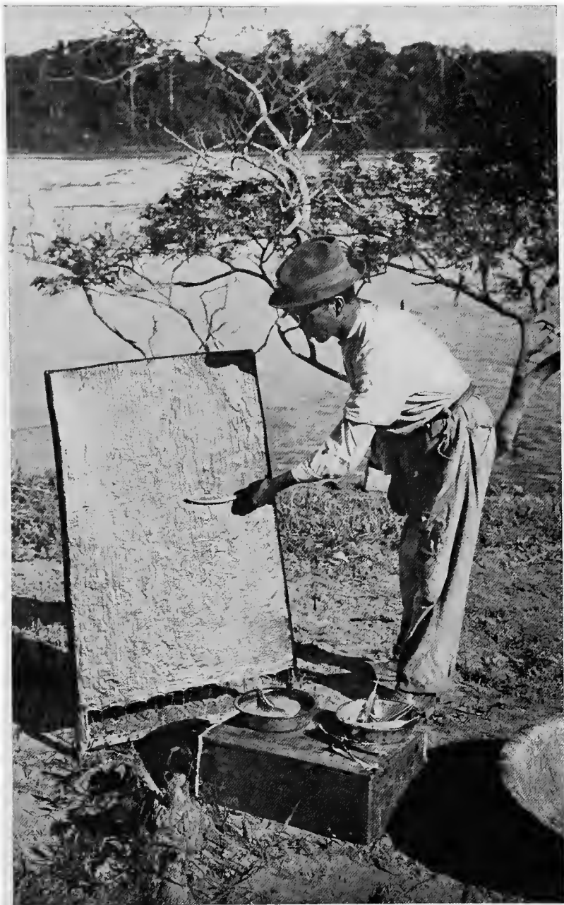
A RUBBER GATHERER MAKING A RUBBER SACK BY COVERING CANVAS WITH LIQUID RUBBER.
