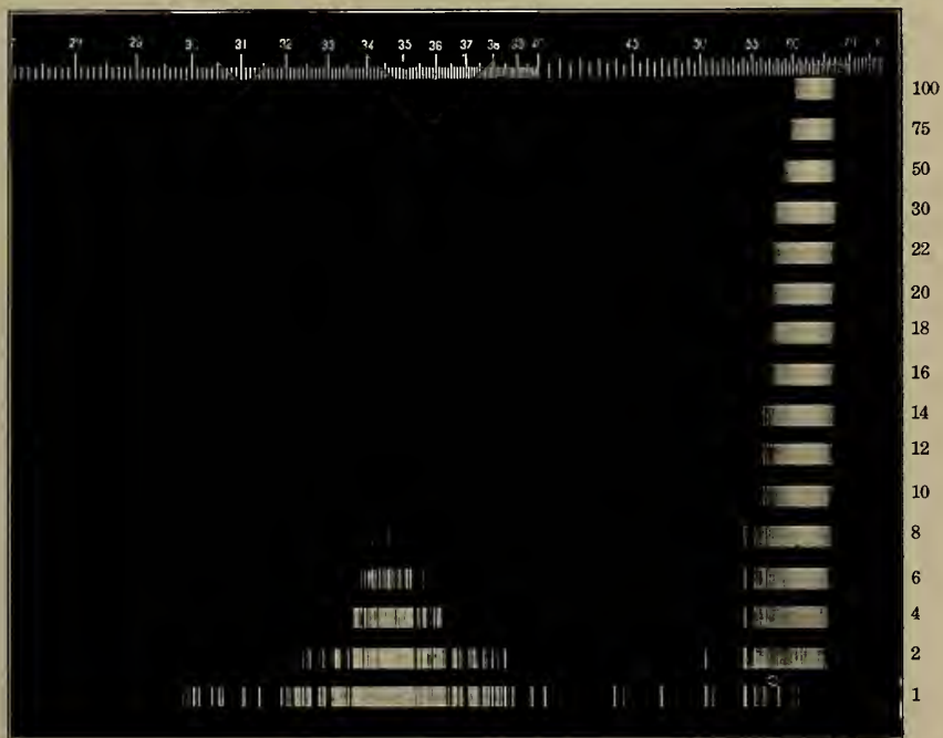
Fig. 1. Potassium salt of white phthaloxime in 90 per cent alcohol. 1/100 molar solution. Thickness of layer, 1, 2, 4, 6, 8, 10, 12, 14, 16, 18, 20, 22, 30, 50, 75, and 100 millimeters.
