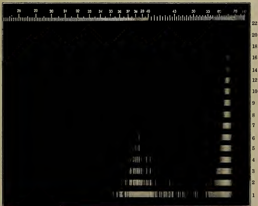
Fig. 2. Silver salt of white phthaloxime in pyridine. 1/100 molar solution. Thickness of layer, 1, 2, 3, 4, 5, 6, 7, 8, 9, 10, 12, 14, 16, 18, 20, and 22 millimeters.
