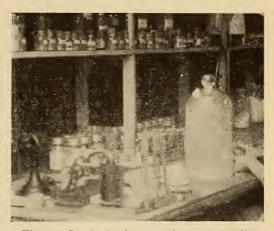
Fig. 1.—In the background is the tall bell jar used as a dusting tower. A charge of dust is suspended in its interior. In the foreground is the mixing-mill used to roll the dust mixtures.
