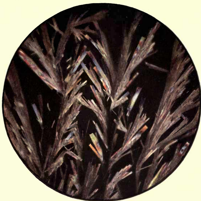
FIG. 99. Salicin. Orthorhombic crystals from alcoholic solution.
