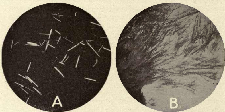
FIG. 126. Menthol: A, individual crystals obtained by sublimation; B, the commonly occurring aggregates of very fine needles.
