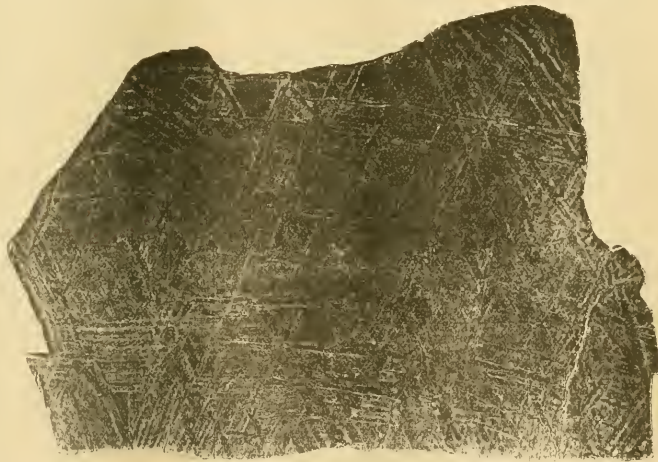
FIG. 2.—The Sacramento Mts. Meteorite. (Printed directly from the etched surface of the iron.)
