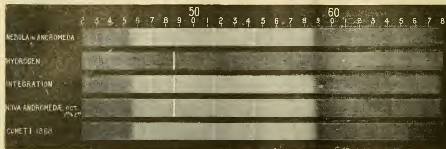
FIG. 2.—Spectrum of the nebula in Andromeda compared with Nova Andromedæ and comet. The flutings common to all are those of carbon.
