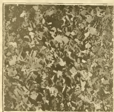
FIG. 2.—Alloy containing copper 30 per cent., zinc 70 per cent., annealed at 700°.
