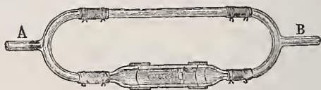
GAULE'S MAXIMUM AND MINIMUM MANOMETER, A, B. (The extremity A is connected with the heart, and B with the mercurial manometer.)
