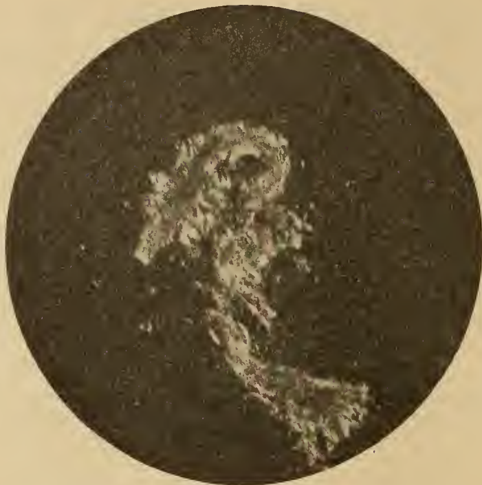
FIG. 10 (magnification \times 180 ).—Photomicrograph of calcium hydroxide-phenol crystals of the unaerated cement recorded in Table IV. It shows the typical plume-like habit of the crystals. Crystalline formations of this character are characteristic of coarse particles of sintered lime which is free from even partial hydration.
