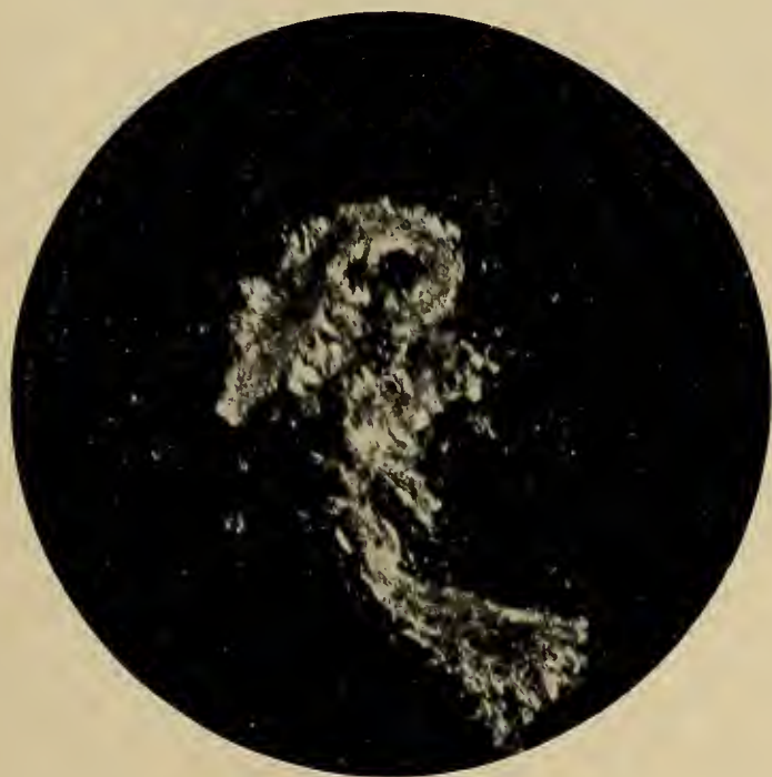
FIG. 10.—Characteristic plume-like formations of crystals obtained from coarse particles of sintered lime in nonseasoned, hard-burned Portland cement.
