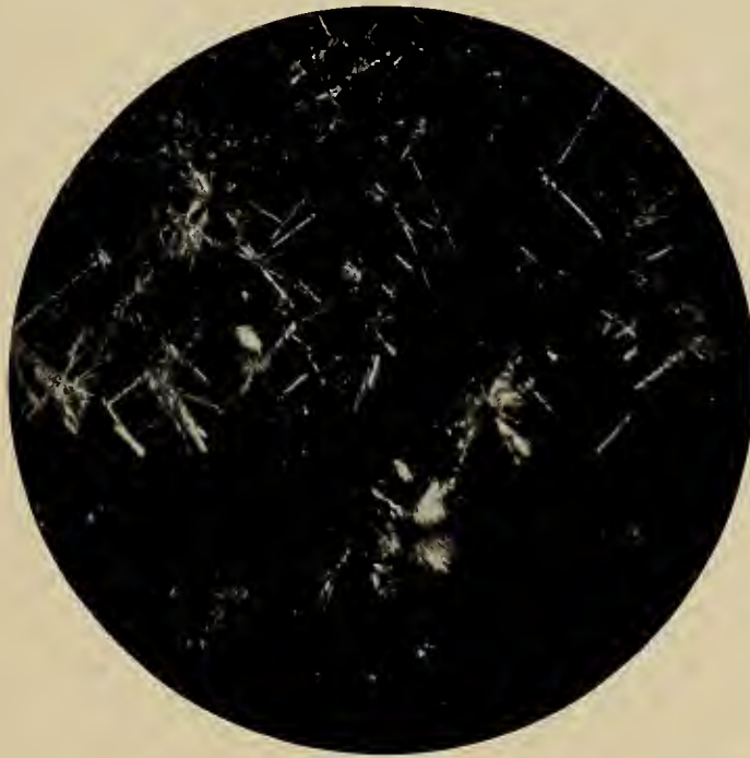
FIG. 11.—Characteristic rosettes of long, slender crystals obtained from the coarse particles of sintered lime in hard-burned cement after they had reached the final stage in the process of hydration by aëration.
