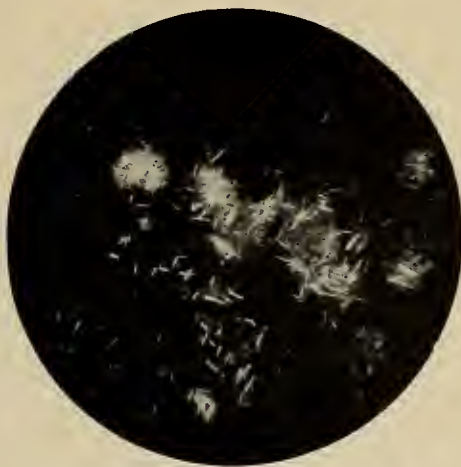
FIG. 5.—Characteristic crystals obtained by the microscopic test from calcium oxide ignited at a red heat.
