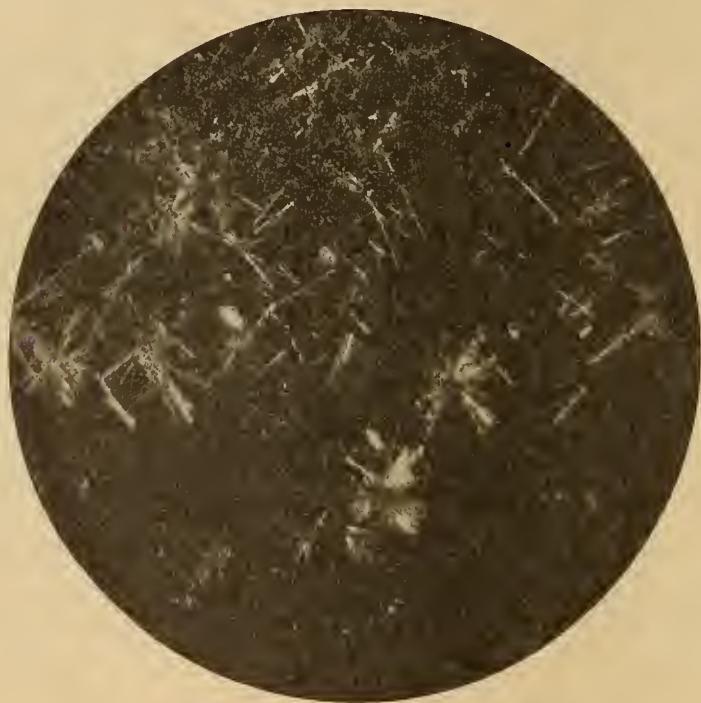
FIG. 11 (magnification \times 180 ).—Photomicrograph of the crystals from the same cement after it had been aerated for eighty hours (see Table IV). It shows the rosettes and the long slender needles which are characteristic of the hydroxide. This figure represents the final stage in the process of hydration of the sintered lime, i. e., the total disappearance of plume-like crystals.
