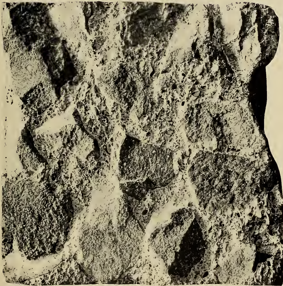
CRUSHED CUBE OF CONCRETE MADE FROM FIRST-CLASS AGGREGATE.
