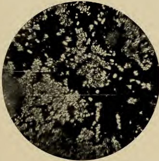
FIG. 4.—Crystalline calcium hydroxide obtained from sintered lime.
