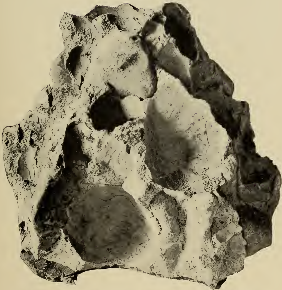
CONE FROM CRUSHED CUBE OF CONCRETE FROM ABATAN RIVER, CORTES, BOHOL SHOWING EFFECT OF USING GRAVEL COVERED WITH GREEN ALGÆ.
