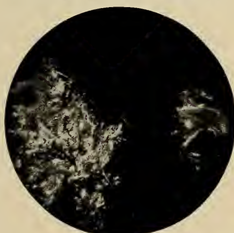
FIG. 7.—Characteristic plume-like formations of crystals obtained from sintered lime.
