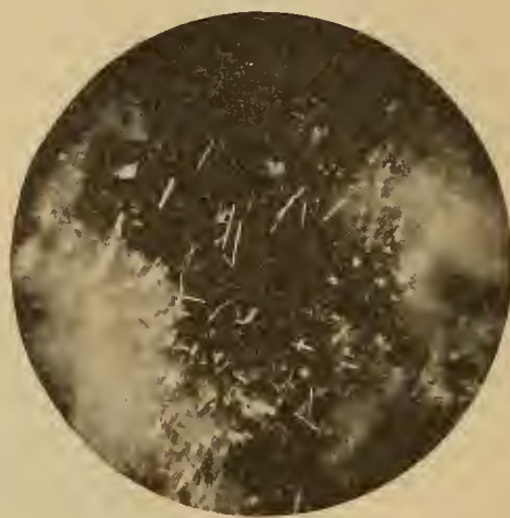
FIG. 6.—Characteristic crystals obtained by the microscopic test from nonsintered lime in Portland cement.
