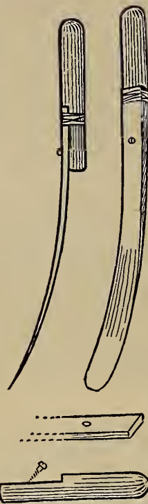
A dibble made from part of an old carriage spring and a broom handle
