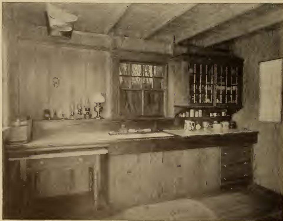
A great deal can be done to lighten labor in the kitchen by making the plan fit the conditions. In this case there is ample work space, and the sink is properly put in the lightest place. The space-saving recess in which the table fits is a novel feature, too.
