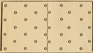
A B 5—Packing 176 to the box; first, third and fifth layers as in A, and second and fourth layers as in B.
