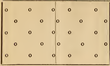
A B 3—Packing 126 to the box; first, third and fifth layer as in A, and second and fourth layer as in B.
