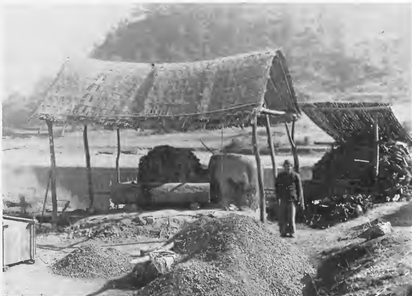
FIG. 1. BACK VIEW OF LEAD BLAST FURNACES IN THE MING-KUAN, (Showing blower).
