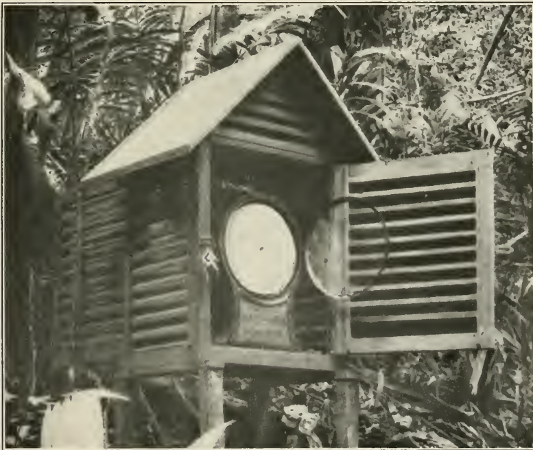
Fig. 6. Station for investigations on plant physiology, Mount Maquiling. Shelter for self-recording hygrometer.
