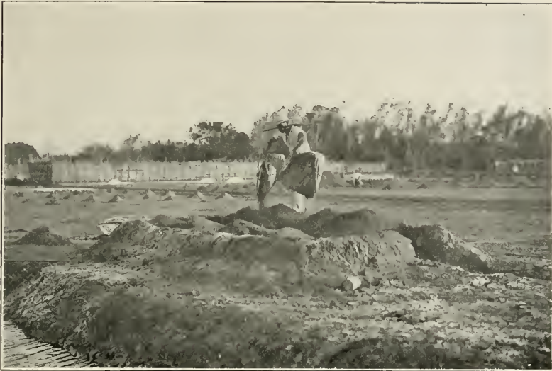
Fig. 1. A leaching vat built on the ground, but high enough so that the mud may be removed by gravity after the leaching is completed.
