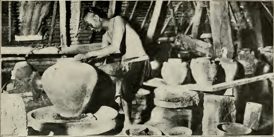
Fig. 1. Finishing a "tenaja."
