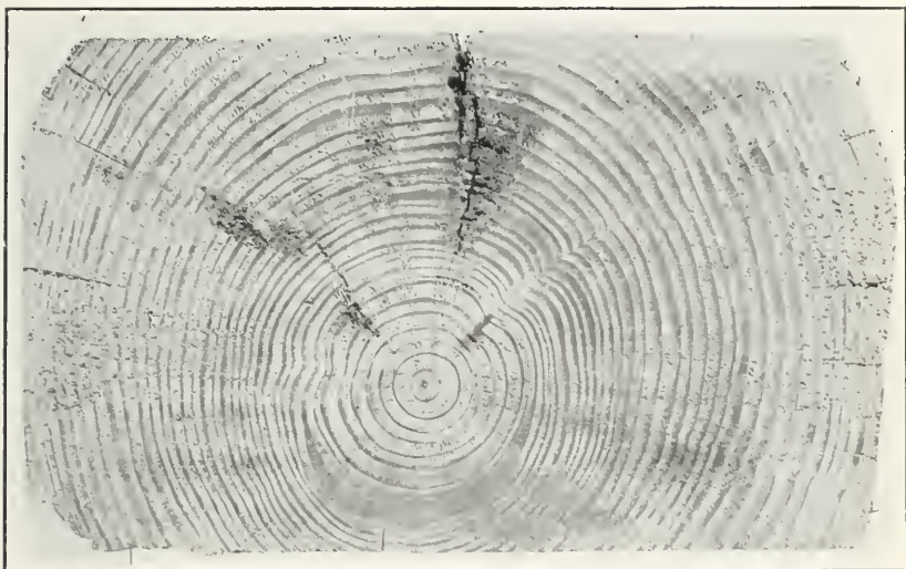
FIG. 1.—EARLY STAGE OF DECAY CAUSED BY LENZITES SEPIARIA.
