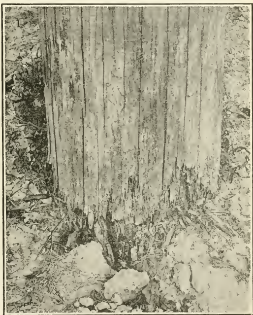
FIG. 3.—Lower end of telephone pole, showing decay at surface of ground while it is practically sound a short distance above.
