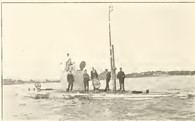
A RUSSIAN SUBMARINE. THREE OPEN HATCHES ARE SHOWN, AND IN TWO COVERS THE DARK LINE OF THEIR THICK RUBBER GASKETS CAN BE SEEN.
