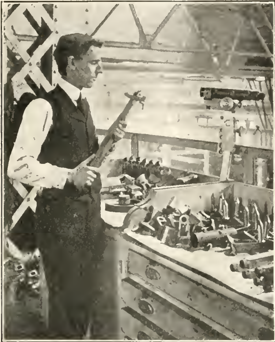
MAKING THE RUBBER CAPPED "EYE" FOR THE GUN POINTER.
