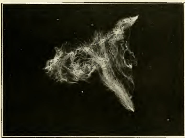
FIG. 6.—THREE-PHASE SPARK-OVER NEEDLES AT ONE MILLION VOLTS, 60 CYCLES, SINE WAVE, EFFECTIVE. NEEDLES ARRANGED IN AN EQUI-LATERAL TRIANGLE APPROXIMATELY 9\frac{1}{2} FEET ON SIDE
