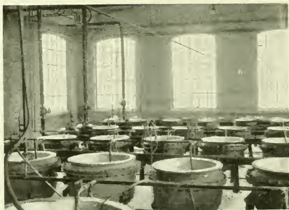
2. ROOM FOR FRACTIONAL CRYSTALLIZATION
