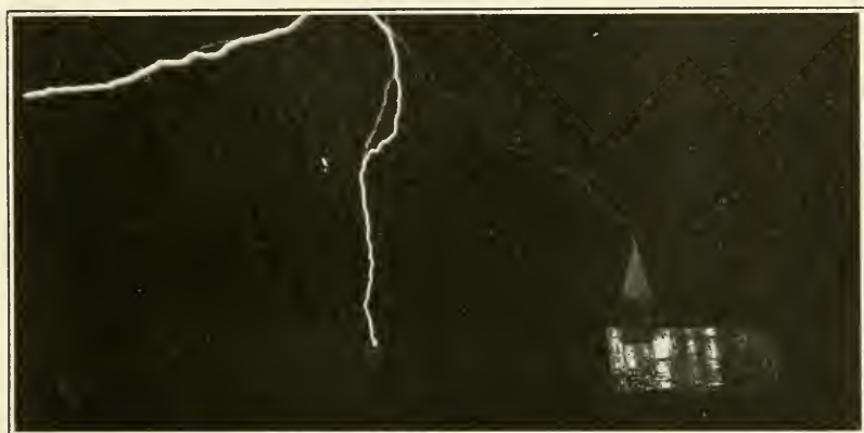
FIG. 39.—ARTIFICIAL LIGHTNING STROKE FROM THE 2,000,000-VOLT LIGHTNING GENERATOR STRIKING HOUSE AND CHURCH OF MODEL VILLAGE DURING STUDY OF LIGHTNING PROTECTION OF BUILDINGS
