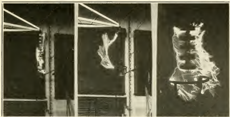
FIG. 27.—SIXTY-CYCLE SPARK-OVER OF SUSPENSION INSULATOR STRINGS
