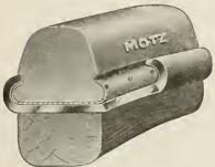
MOTZ MOTOR BUGGY TIRE. [Clincher type. Held in rim by steel cross bars placed slantwise in the hase of the tire, the ends of the bars extending under the flanges of the rim. Motz Clincher Tire and Rubber Co., Akron,
