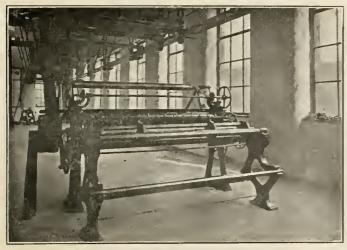
RIPPING MACHINE FOR BELT SLITTER.
