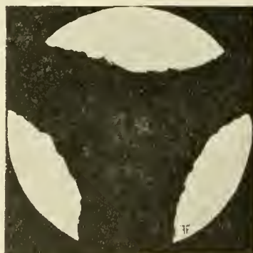
FIG. 7.—Intersection of three cells—section through the middle of the lump on the line C D, Fig. 4.
