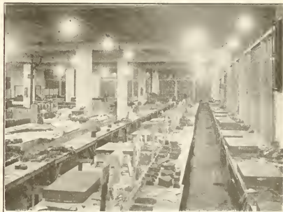
FIG. 6. TYPICAL OVERHEAD ILLUMINATION OF UPPER-CUTTING ROOM, ELIMINATING SHADOWS.
