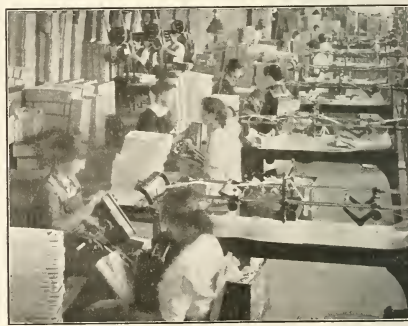
FIG. 2—MACHINES FOR PAPER-COVERING CARTONS.
