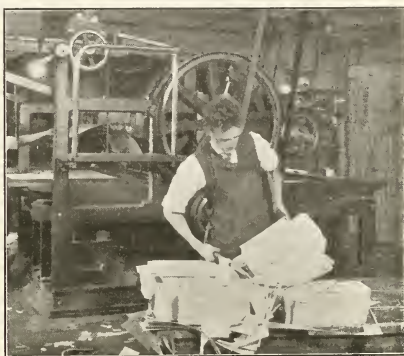
FIG. 4—PRESS FOR CUTTING, SCORING, AND PRINTING CARTONS.
