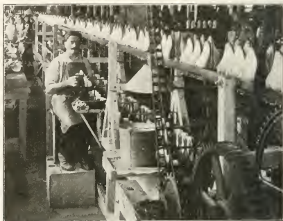
CEMENTING AND DRYING CEMENT ON CONVEYOR BELTS.
