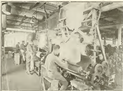
FIG. 4.—ELECTRICAL RUBBER FABRIC TESTING MACHINES.
