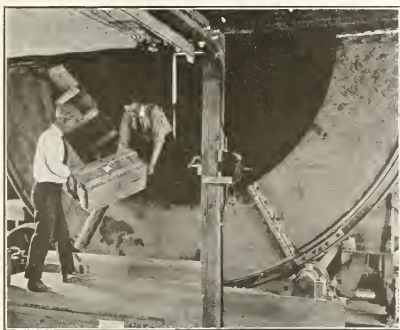
EXTERIOR VIEW OF 14-FOOT DRUM BOX-TESTING MACHINE.
