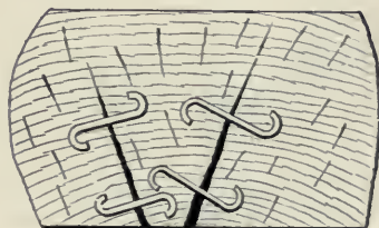
FIG. 78.—Method of using "S" irons to prevent the further opening of checks in cross ties.
