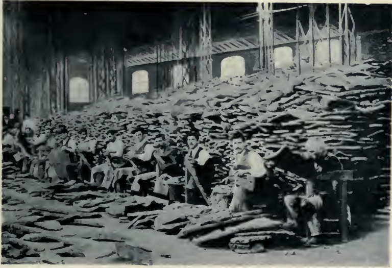
FIG. 119.—Sorting and trimming sheets of cork. The best grades are used for bottle stoppers.
