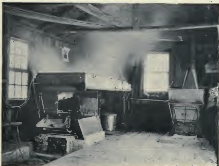
FIG. 105.—Interior of a sugar house showing the steaming evaporator at the left and the "sugaring-off" arch at the right.
