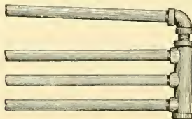
1000. Pipe work for modern greenhouse heating. A wall coil.
