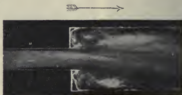
FIG. 13.—Sudden enlargement (thick sheet.)
