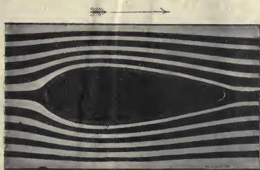
FIG. 9.—Section of screw shaft strut (broad colour bands in thin sheet).
