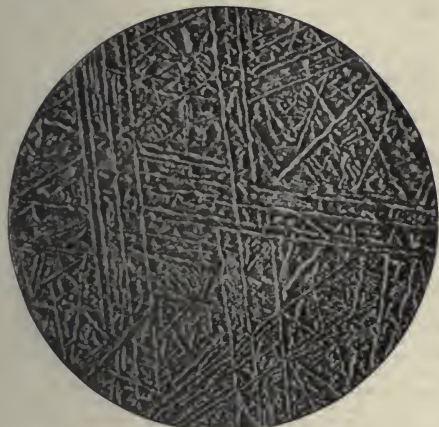
FIG. 1.—Silver-lead eutectic, \times 100 . Oblique illumination.
