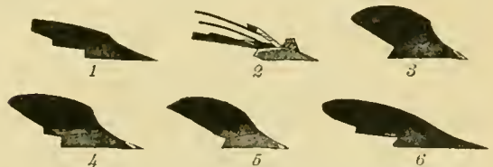
2251. Types of moldboard plows adapted to different kinds of plowing: 1, prairie breaker bottom; 2, rod breaker bottom; 3, stubble bottom; 4, general-purpose bottom; 5, black land bottom; 6, tame sod breaker bottom.
