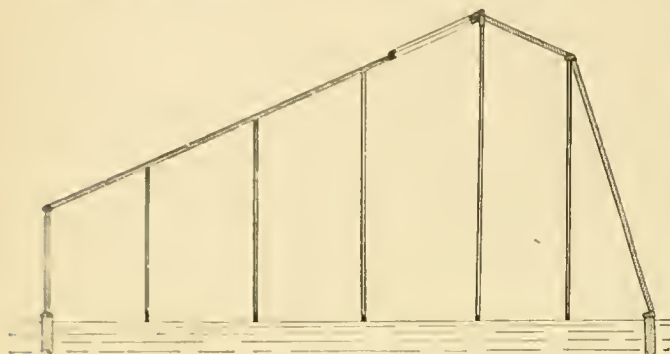
2148. Showing type of greenhouse constructed to obtain the maximum amount of light in short winter days. Modification of type shown in Fig. 2147. Obstructs more light than Fig. 2147, but could be built wider.
