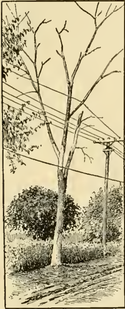
Fig. 50. Elm tree killed by a direct current from an electric railroad system.
