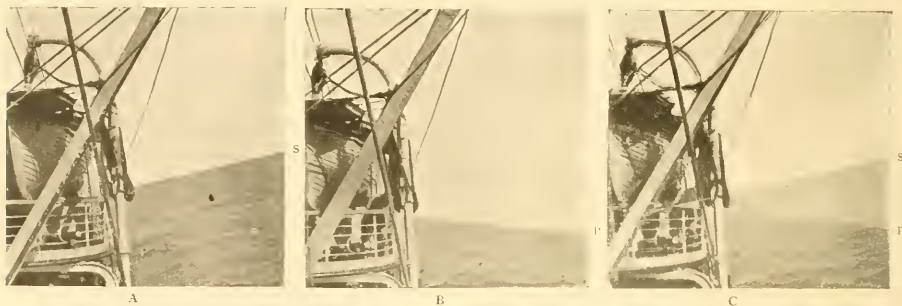
Union Steamship Co's Mokoia . Rolling angle found by photography. A is a picture taken at the instant of the end of rolling to the right, B is a picture taken at the end of rolling to the left, C is a composite picture made by superposing the two films, A and B. The pictures of the ship are made to coincide, thus the angle between the two horizons in A and B is found. Lat. 34° 27' S. Long. 157° 45' E. To Sydney 325 miles.
