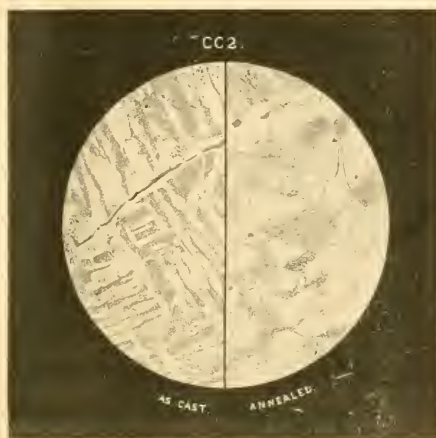
FIG. 1.—Casting CC2. (Reduced from six-inch circle, magnified 315 diameters.)
