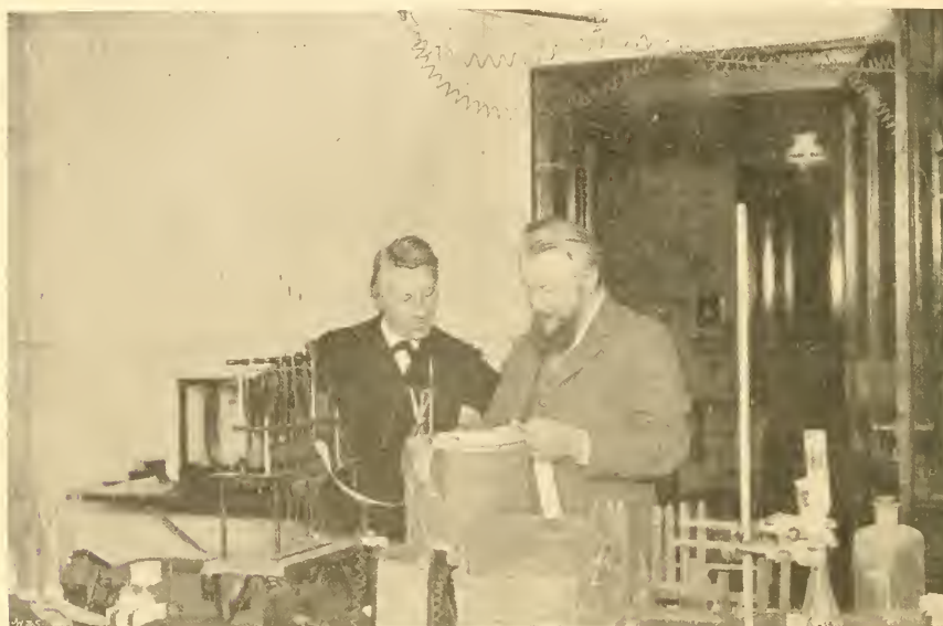
FIG. 1.—Ostwald and van't Hoff. (Taken in Ostwald's private laboratory.) The illustration shows the two investigators standing by Prof. Ostwald's apparatus for automatically registering on a strip of paper the peculiar phenomena attending the solution of metallic chromium in acids.
