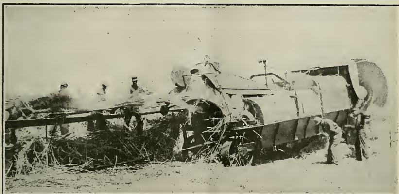
FIG. 1.—Hemp-breaking machine. The stalks are fed sidewise in a continuous layer 2 to 3 inches thick, turning out about 4,000 pounds of clean fiber per day and five times as much hurds.
