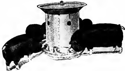
FIG. 74.—The "hog motor," a device for making pigs grind the corn they eat. (Hog Motor Company, Minneapolis.)
