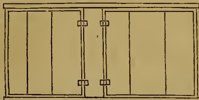
Fig. 2.—South side of span. The sashes, lifting on hinges, give ventilation at top, bottom, and ends.
