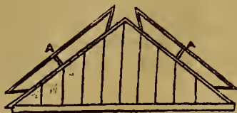
Fig. 1 shows the east end, one sash on the south side, and one on the north side, being tilted. A A are two chocks, which tilt the sashes. The sashes are hinged on the other side.
