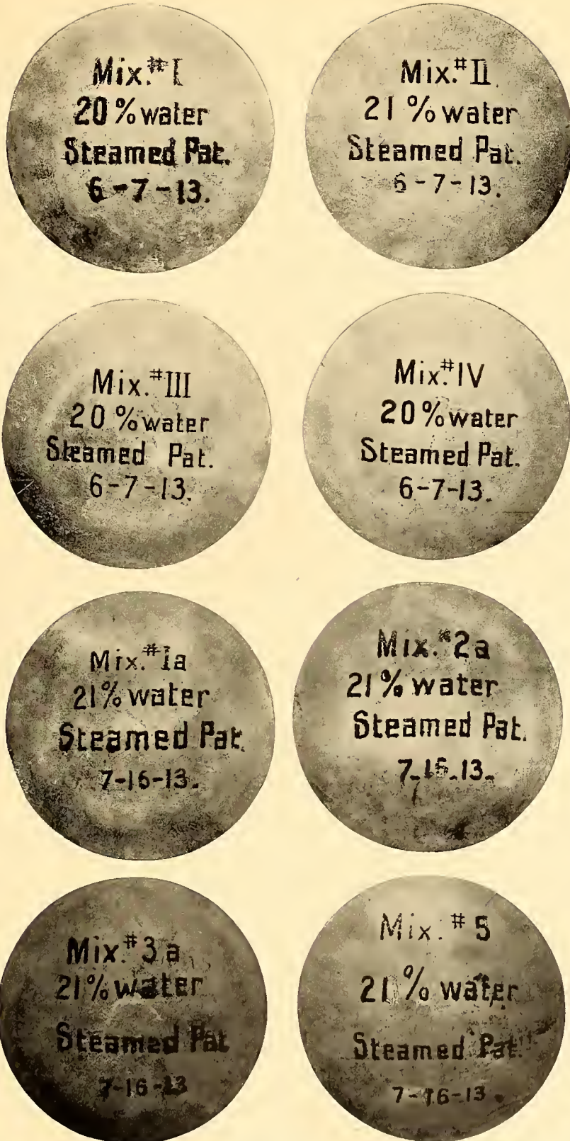
PLATE I. SOUNDNESS PATS OF NAGA CEMENT AFTER FIVE-HOUR STEAMING TEST.
