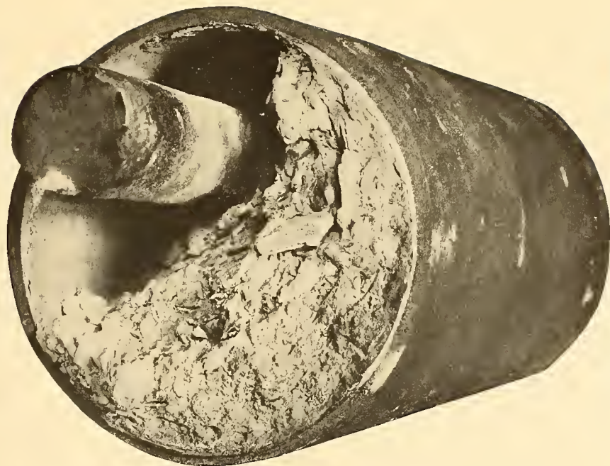
Fig. 2. Section of the same tube, showing an iron cleaning rod broken off in an attempt to remove the scale.
