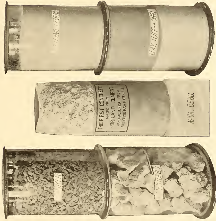
Fig. 1. Raw materials from Naga, Cebu, and the Portland clinker, cement, and concrete produced.
