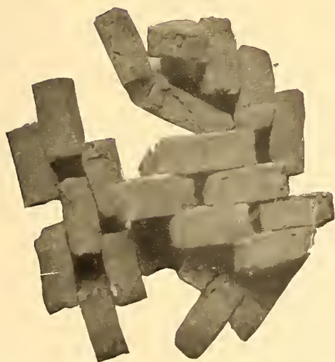
Fig. 2. Perfectly sintered Portland cement clinker made from available Philippine raw materials and burned in our experimental kiln.
