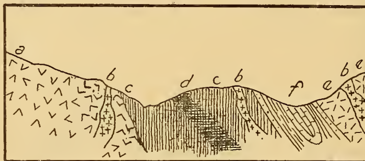
FIG. 6. Geologic section through ore body at Hison, along an east-west line; diagrammatic in part: (a) Granite; (b) intrusives; (c) altered wall rock; (d) iron ore; (e) effusives; (f) limestone, shale, and sandstone; length of section, about 200 meters.
