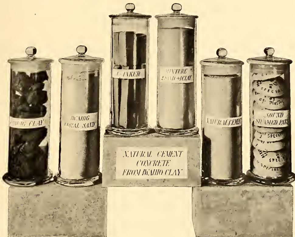
Fig. 2. Iwahig raw materials and the natural cement products obtained from them.
