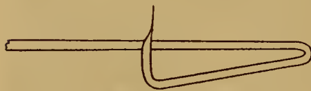
FIG. 14. Special pipette for measuring small quantities of liquid.
