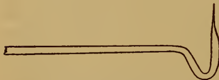
FIG. 11. A pipette constructed for use above a barrier of blotting paper.
