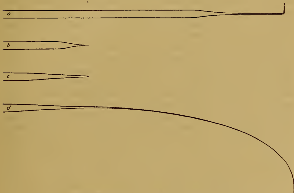
FIG. 6. a , Completed pipette; b , c , and d , various sorts of points.
