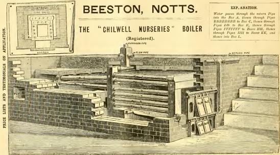
We can CONFIDENTLY RECOMMEND THIS BOILER for Heating Apparatus of 1500 feet and upwards. We have had a number of these Boilers at work for five years, and THEY HAVE GIVEN GENERAL SATISFACTION. IAL SATISFACTION. The Boilers are now also made with 2-INCH WROUGHT WELDED STEEL TUBES, which diminish the risk of breakage. THEY HAVE STEEL WATER RARS.
